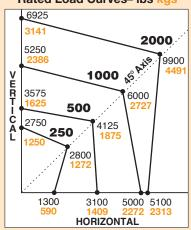
Horizontal, Vertical and 45° plotted Ratings are California OSHPD submitted values having the OSHPD Anchorage Preapproval Number OPA-0196. Testing and calculations were performed to meet OSHPD criteria.
